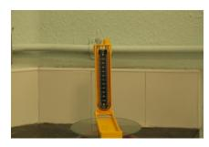
3. Based on a calibration experiment, each unit on the manometer scale corresponds to a volume of 15.85mm³ in the manometer tube and there is 640 mm³ of tube above the scale on each side of the Utube. Hence, the volume of trapped air will be, in cubic millimetres,
