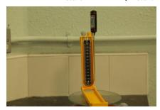
4. Strap the digital thermometer adjacent to the U-tube with some tape without obstructing manometer scale or the fluid level in the tube. Record the temperature and then place the manometer with putty and thermometer in the refrigerator.
