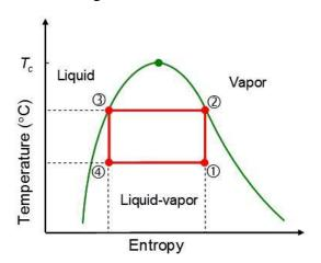
Discuss the fact that the power cycles in the previous two chapters (lessons) go around this ideal cycle clockwise where as for a refrigeration cycle it is necessary to go around anti-clockwise.
