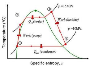
State 3 (input to turbine):  $P_3 = 15000 \,\text{kPa}$ ,  $T_3 = 600 \,^{\circ}\text{C}$ , so using the steam tables  $h_3 = 3579.7767 \,\text{kJ/kg}$  and  $s_3 = 6.6764 \,\text{kJ/kg/C}$
