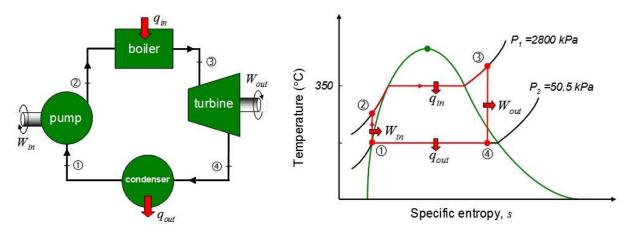
State 4:  $P_1 = P_4 = 50.5$  kPa and  $s_4 = s_3 = 6.7842$  kJ/kg/C which corresponds to a saturated mixture. In order to find the quality of the mixture we need from the steam tables,  $s_f = 1.0941$  kJ/kg/C and  $s_{fg} = 6.4972$  kJ/kg/C
