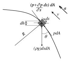
Note that Bernoulli's equation can be expressed such that the terms have the units of pressure by normalizing with density,  $\rho$ ; or of length or head by normalizing with gravitational acceleration, g. Thus, piezometric head can be defined as  $(p/g\rho+z)$ ; total head as  $(v^2/2g+p/g\rho+z)$ ; and stagnation or total pressure as  $(p+\rho v^2/2)$ .
