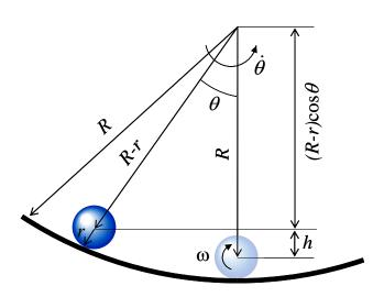
The potential energy gained when the ball is displaced from bottom of the bearing is:
