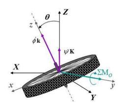
This is the couple that must be applied to maintain the steady precession, i.e.  $\dot{\theta} = \ddot{\psi} = \ddot{\phi} = 0$  assuming that the center of gravity of the wheel is fixed in space ( $\Sigma F=0$ ).
